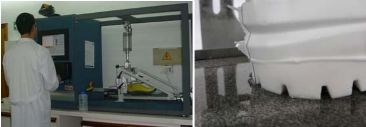
Figure 3 : Images of experimental phase Figure 3.1 : Slip testing Figure 3.2 : Detail of a sole sample being tested
